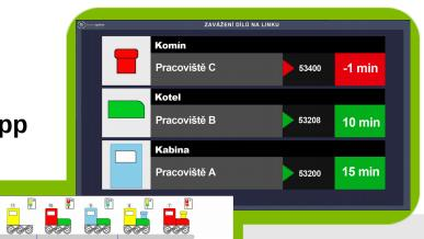
Based on product configuration, consumption of particular part variants and materials on individual workstations is recorded by the system.
